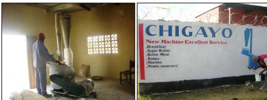
The hammer mill machinery is very expensive but very worthwhile. This is the first major income generating project for NBCV. The equipment is used like this. The hammer mill grinds corn seed into fine meal locally known as mealie- meal from which our main dish nshima is prepared. The maize de – huller processes or peels off the corn grain to make a grit product known as sampo or cleaned broken pieces of maize suitable for a breakfast cereal. The de huller also processes the corn seed into semi
